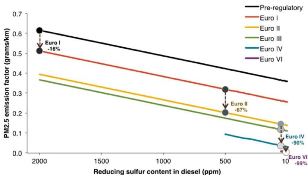
Figure 1.2. Impact of fuel sulfur levels and emissions control standards on PM<sub>2.5</sub> emissions from heavy-duty diesel vehicles (grams/km)
